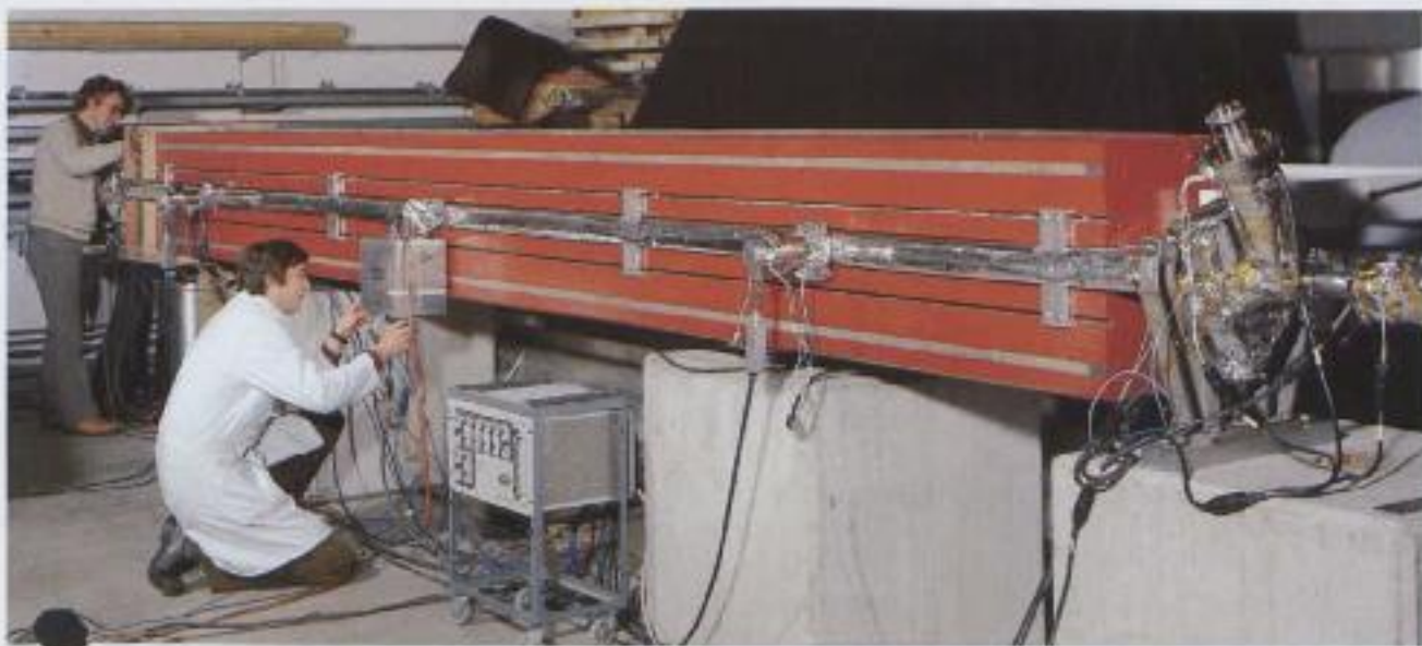
A prototype magnet for LEP which has been built with the new technique of spacing out the steel laminations and filling the gaps with mortar. This is acceptable because only low magnetic fields are needed. Such magnets provide adequate fields at half the cost of conventional magnets, and have better mechanical properties.
