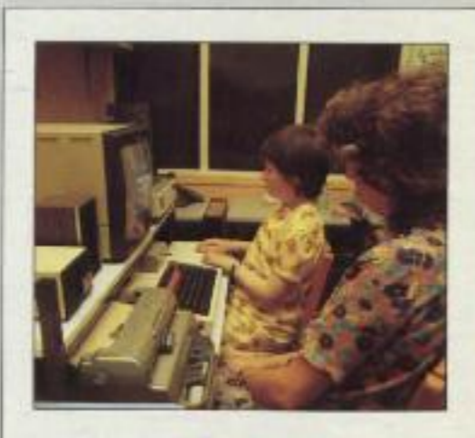
Learning to read with technology – a young girl uses a synthetic speech system to learn braille. It 'speaks' letters as they are typed on the Perkins Braille or the computer keyboard, and can read back the text as words or sentences. Reading braille is practised using the Concept Keyboard. Teachers use the monitor screen to check progress.
