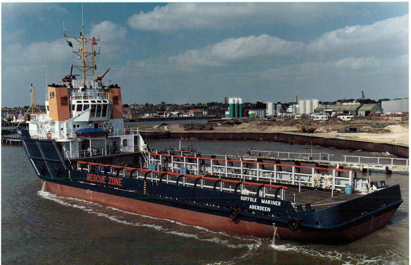
A platform supply vessel which supports offshore drilling rigs and production fields.
