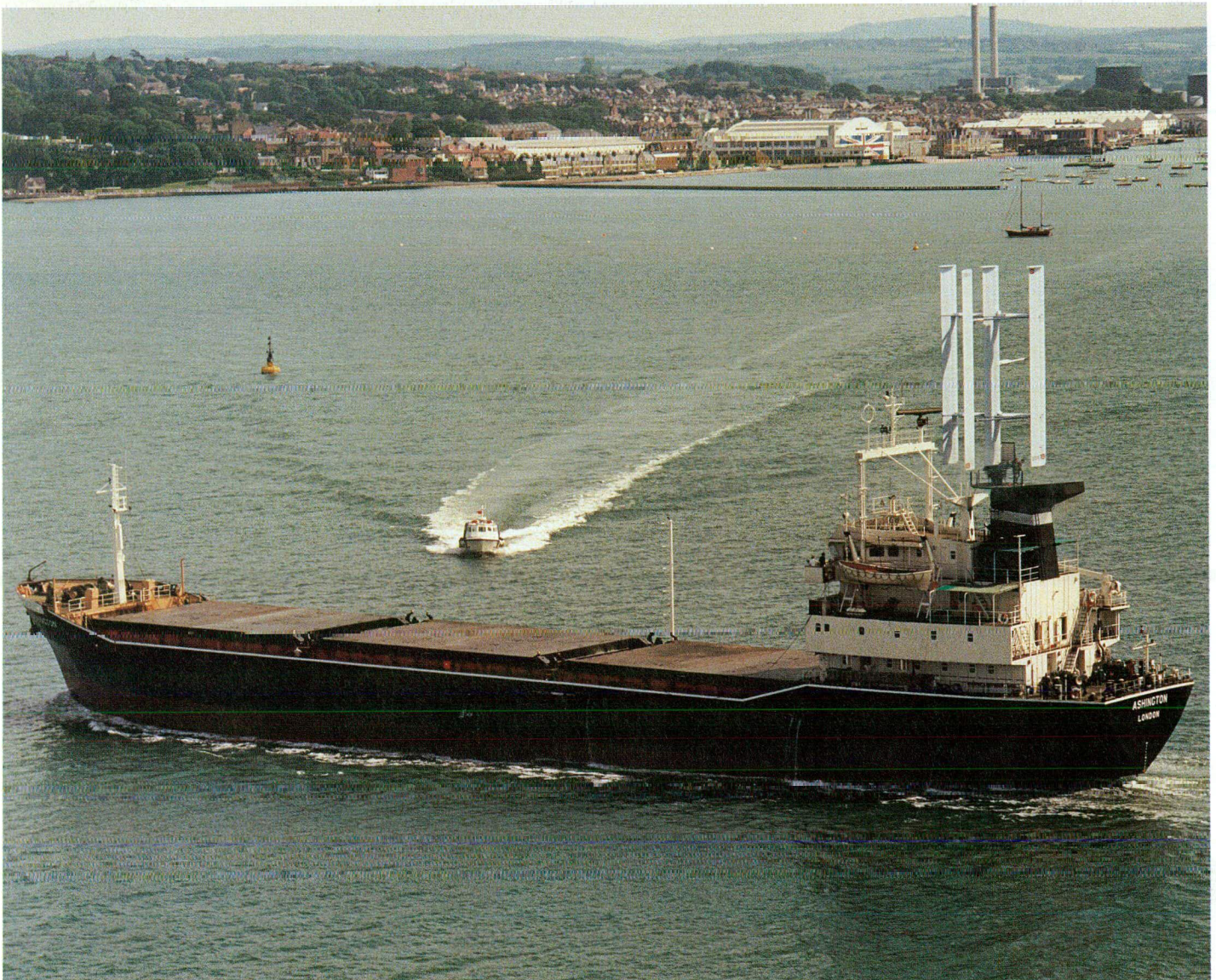
The first British ship to be fitted with advanced auxilliary sail power, pictured in the Solent.
